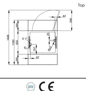
Electric Supply voltage: 220-240 V/1N ph/50/60 Hz Electrical power, max: 2.32 kW Water: Drain line size: 3/4" Key Information: N° of doors: 1 External dimensions, Width: 770 mm 1180 mm External dimensions, Depth: External dimensions, Height: 1304 mm Net weight: 94.5 kg Shipping height: 1334 mm Shipping width: 810 mm Shipping depth: 899 mm Shipping volume: 0.97 m<sup>3</sup> +85 / +95 °C Set temperature: **Sustainability**
